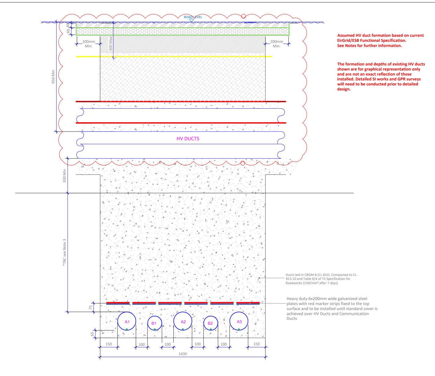
A = 160mm OUTER DIAMETER HDPE ESB APPROVED POWER DUCT, SDR= 21 B = 125mm OUTER DIAMETER HDPE ESB APPROVED COMMS DUCT, SDR=17.6
